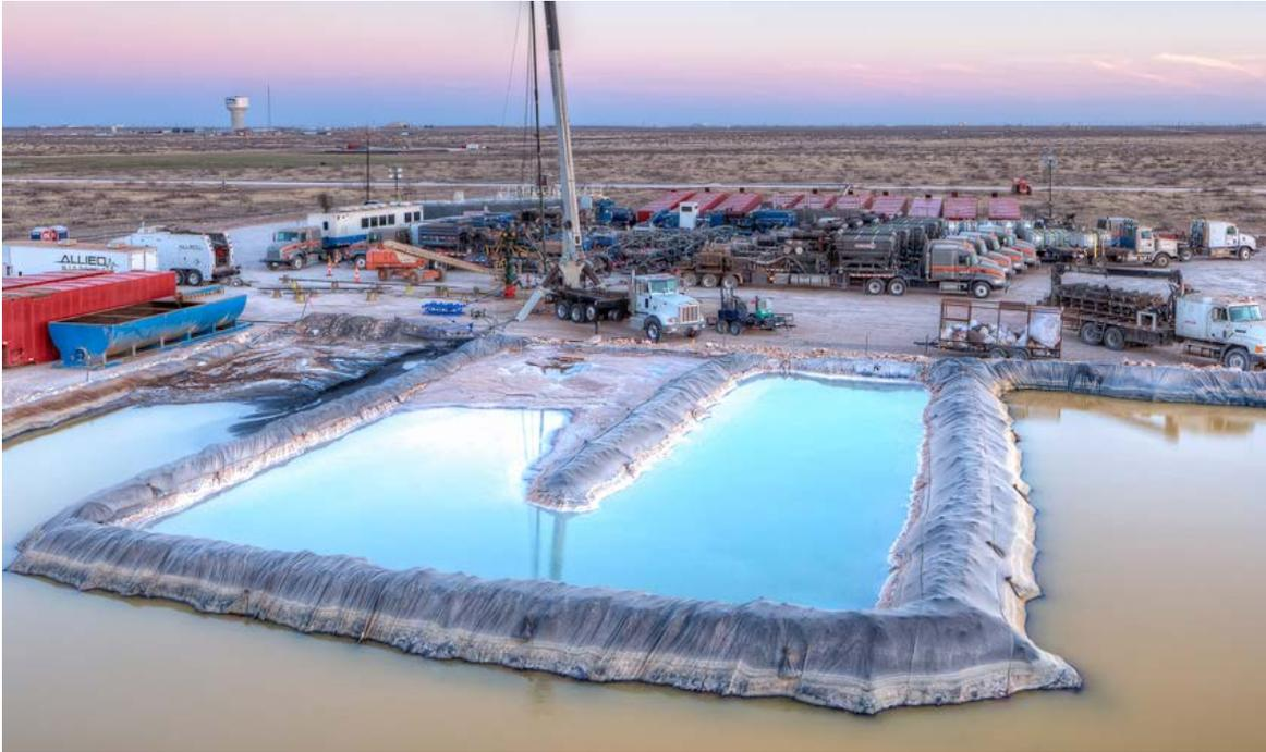
Water is a critical component for well completion, for both pumpdown and frac fluid. Water is such an integral part of upstream oil & gas, that operators often joke about being water companies who produce oil & gas.
